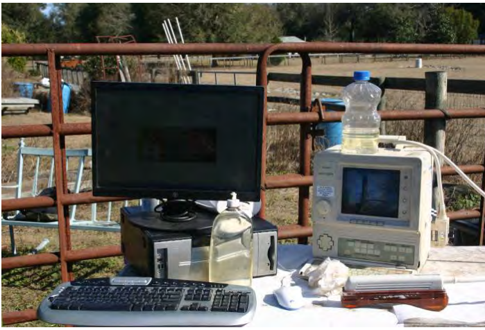
Figure 2. Real-time ultrasound machine, probe, and accessories. Credits: Mark Shuffitt
