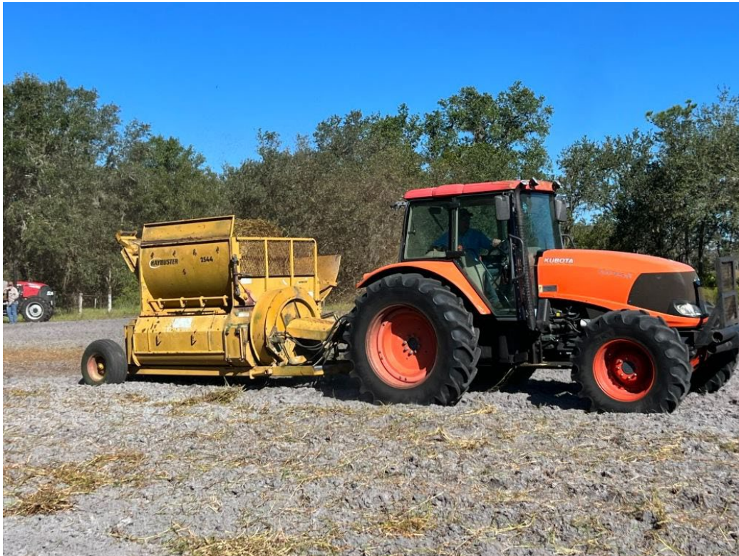
Figure 3. Haybuster used to plant vegetative material (photo by Bridget Stice)
