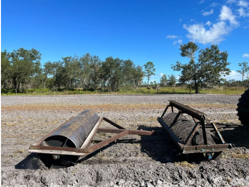
Figure 2. Crimper or 'pizza cutter' used to push planting material into soil with a roller behind it to firm the soil. A second rolling in a perpendicular direction is required (photo by Bridget Stice).
