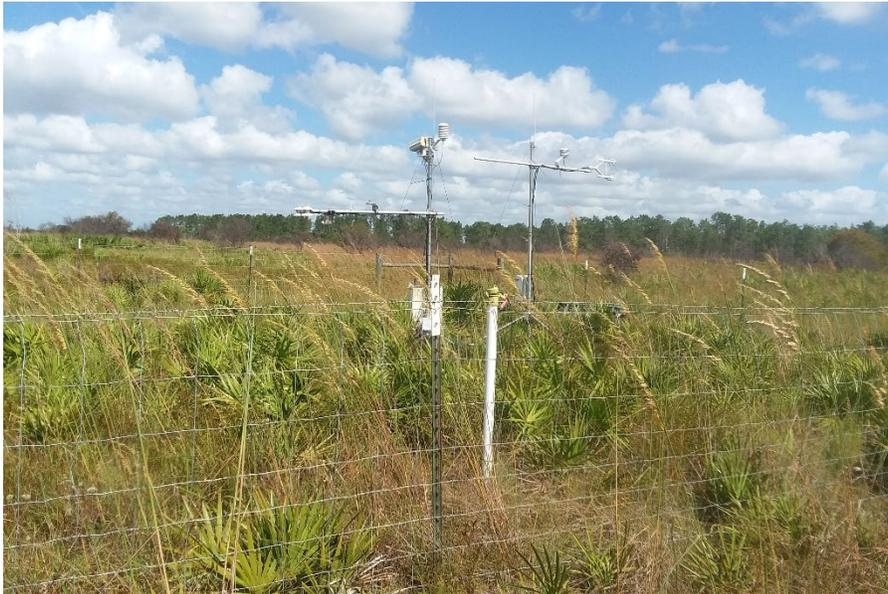
**Figure 4.** Eddy Covariance Tower located at the Range Cattle REC LTAR experiment. This equipment was acquired in 2016 and has been continuously collecting data on ecosystem carbon and water flows, water table depth, temperature, soil radiation, rainfall, wind speed and direction every 30 minutes.
