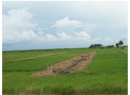
Field layout of stargrass plots at Butler Oak Dairy showing ditch and samplers for collecting runoff groundwater.
