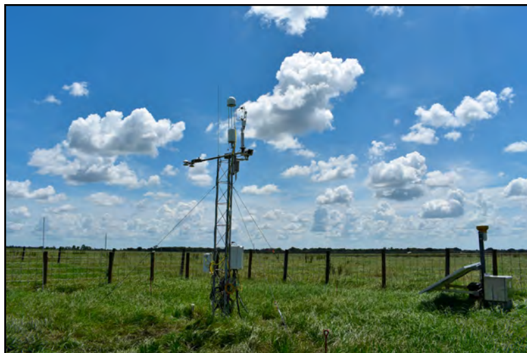
Eddy covariance tower measuring ecosystem carbon fluxes on a bahiagrass pasture.
