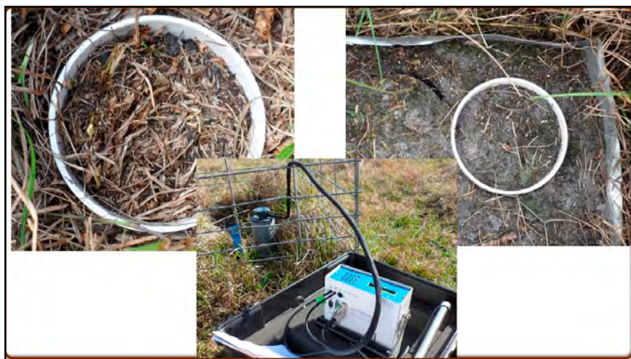
Portable infrared gas analyzer used for soil respiration measurements.
